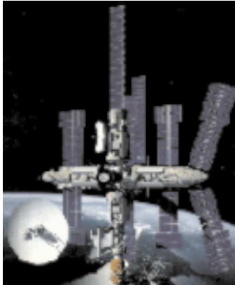
Fig. 4. A solar dynamic system alongside with PV panes for power generation on the international space station Mir (NASA artist's rendition).
