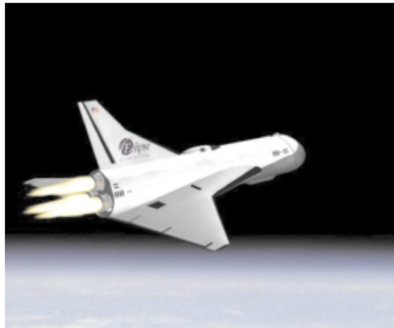
Fig. 13. Astroliner, a reusable space transport vehicle under development by Kelly Space and Technology Co. [69].
