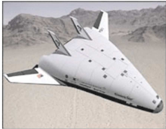
Fig. 15. The X-33 technology demonstrator for full-scale commercially developed reusable launch vehicles. 23 m long, 26 m wide, \text{LH}_2/\text{LO}_2 fueled, it is unpiloted, to take off vertically like a rocket and land horizontally; maximum speed Mach 13+ [61–63].
