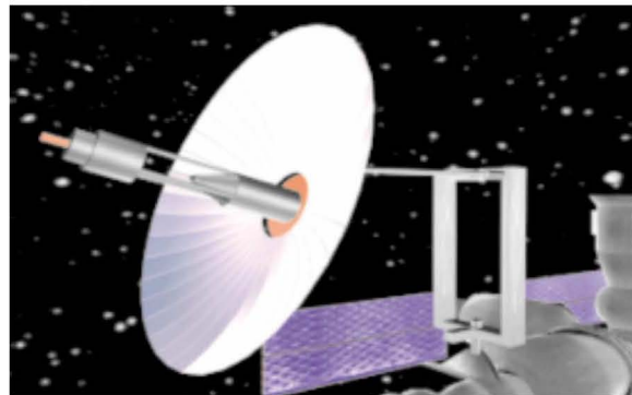
Fig. 3. A solar dynamic concept for space power production: note concentrator and receiver (NASA artist's rendition).
