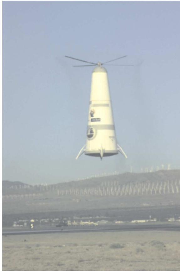
Fig. 14. The Roton-C9, a reusable space transport rocket under development by Rotary Rocket Co. [70].
