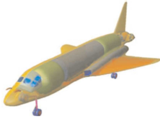
Fig. 12. Pathfinder, a reusable space transport vehicle under development by Pioneer Rocket Plane Co. [68].
